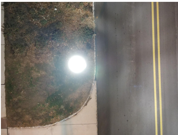
The new Witherspoon light, photographed from directly above by a levitating drone, demonstrates the spill in the night sky.
