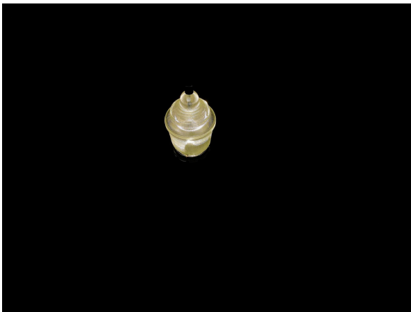
Ultrashort exposure (1/1000th sec) photos to measure the light emission pattern of the fixture. This is the 135° view (45° above horizontal).
