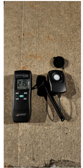
(A) Shoebox LEDs on high poles. Generally overlit, and the lighting is homogenous due to the high poles. 3.59 FC directly beneath the pole and 2.15 FC between the poles, respectively. (Desired value 0.3 FC).
