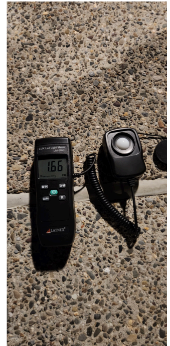
(E) The walkway is excessively illuminated, with both roadway and sidewalk fixtures operating at light levels far higher than necessary, 3.47 FC beneath the pole and 1.66 FC between poles, respectively. (Desired 0.3 FC).
