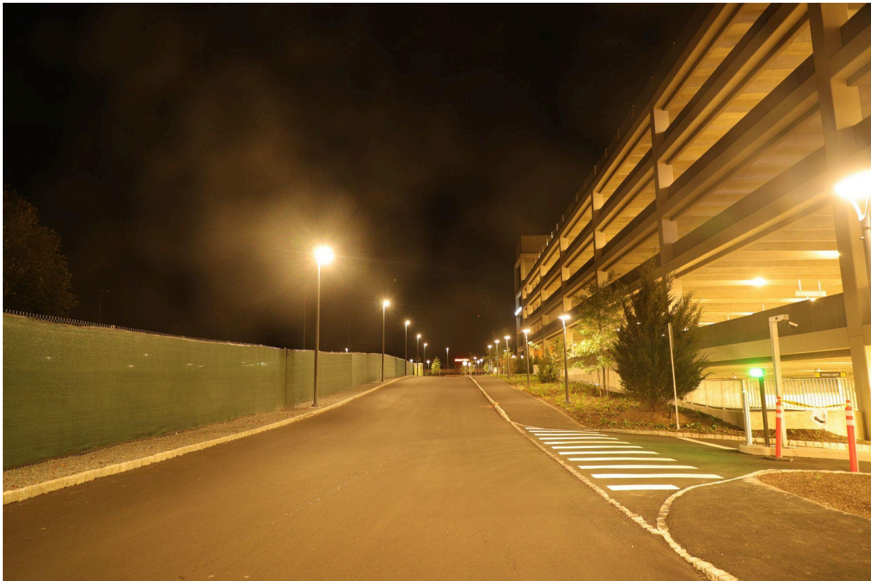
Overlighting and > BUG-0-0-0 fixtures on Stadium Drive spill light in the lakeside woods. See the next image.
