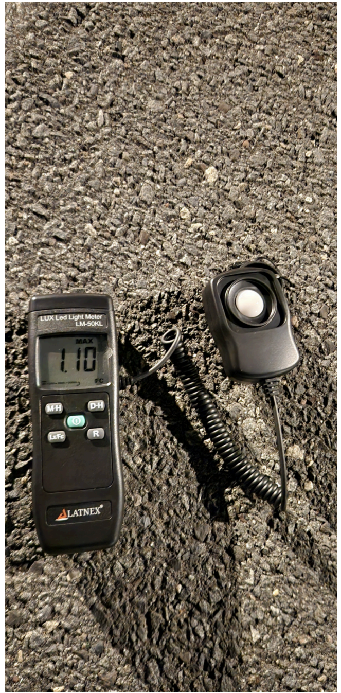
(E) Dimmest point of the dinky parking lot, point furthest from all poles, 1.1 FC measured.
