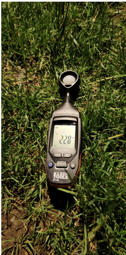
(A) cont. Penn globes, measured at 0.62 FC between poles and 2.28 FC beneath the pole, respectively. (Desired value 0.3 FC).
