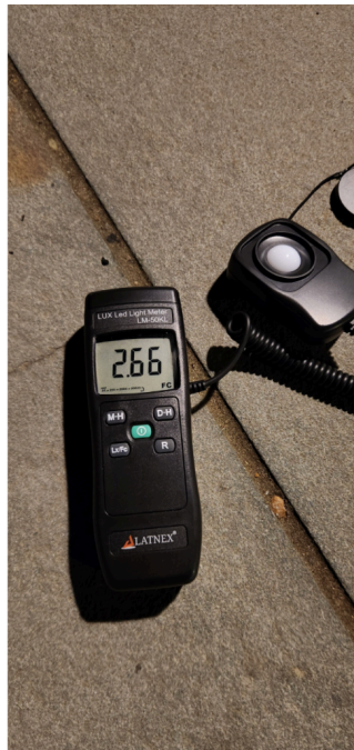
(B) Overall, slightly overlit area. 2.6 FC directly beneath the pole, 0.47 FC between the poles, respectively. (Desired 0.3 FC).
