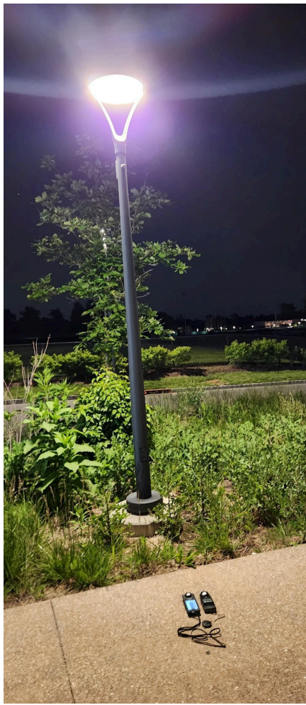
Illuminance measurements on the sidewalk at Stadium Drive, under the fixture, comparing the Sekonic C-800 with the Minolta illuminance meter. The two meters measure illuminance to within 4%.
