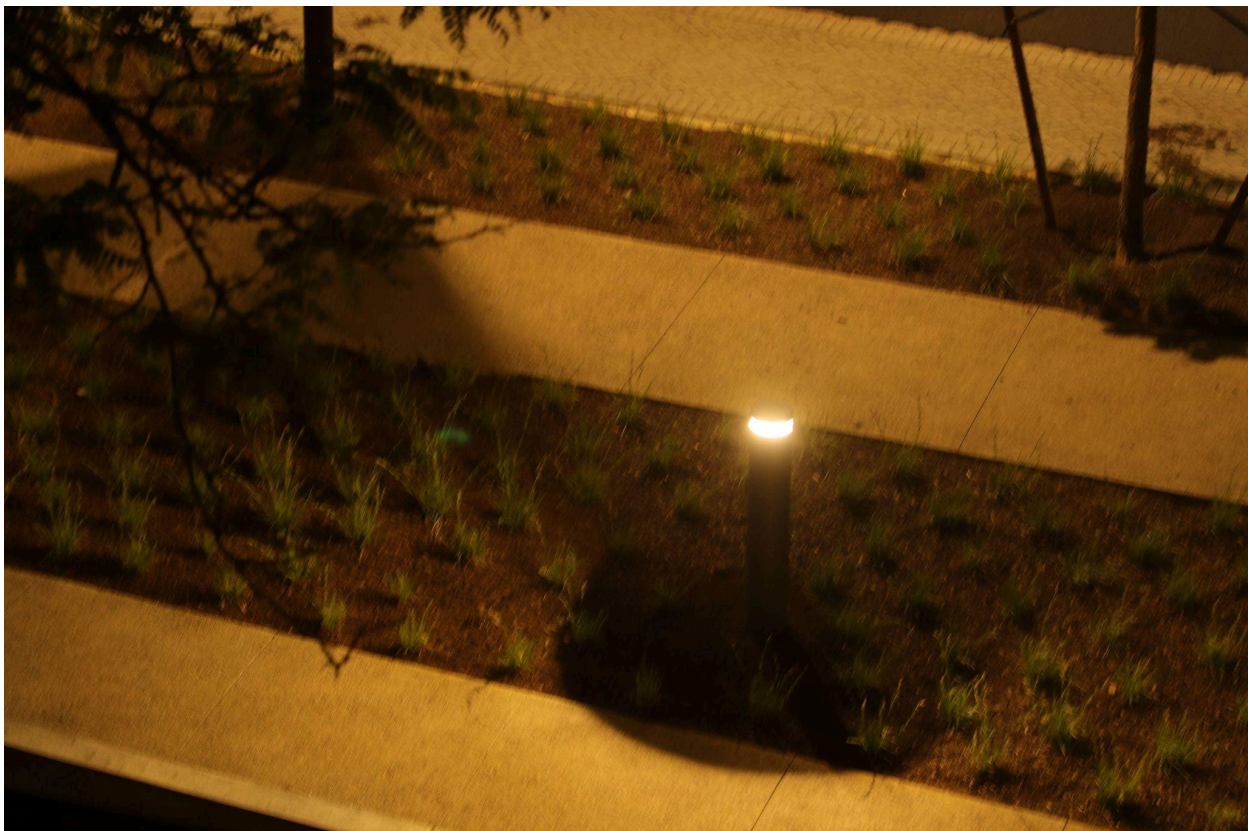
New, unshielded bollards cast light on the roof of Peyton and cause overall glare. Previously used bollards around Peyton BUG ratings with no uplight. Switching to these new ones is a step back.
