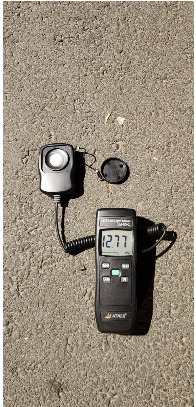
(D) Makeshift LEDs for the walkway. Extremely bright, causing the loss of dark adaptation for other areas that are ~ 10x less lit, 12.77 FC measured.
