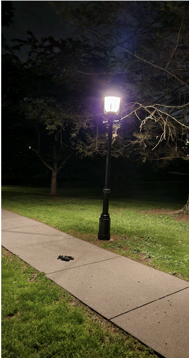
(C) Path from parking lot to graduate college, Penn globes, brighter beneath post, lower but still acceptable limit between posts. Light spills into the nature area. 1.81 FC & 1.66 FC measurements with two different detectors to check for consistency.
