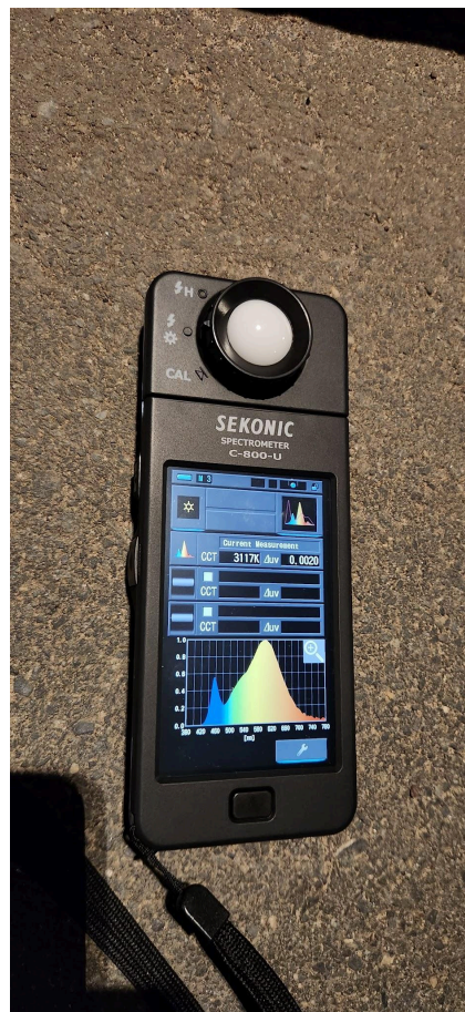
Bega 84* and Bega 99* emission: broad spectrum peaking at an equivalent temperature of 3100K, strong blue peak hiding in the red end.
