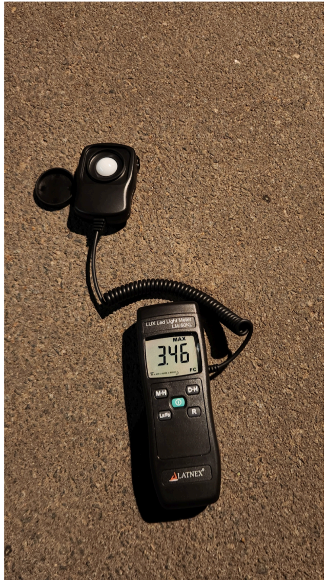
(A) cont. Southside of Peyton Hall, directly beneath the lamp. Measurement of 3.46 FC (target 0.3 FC).
