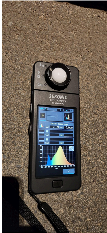
Spectrum of the roadway light. Peaks at 590nm, with a significant blue peak at 400nm.
