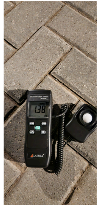
(F) Bright white streetlights, overlit by factors of many, 3.10 FC beneath the pole and 1.38 FC between poles, respectively.
