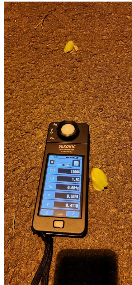
Lighting level under the fixture is 6FC.
