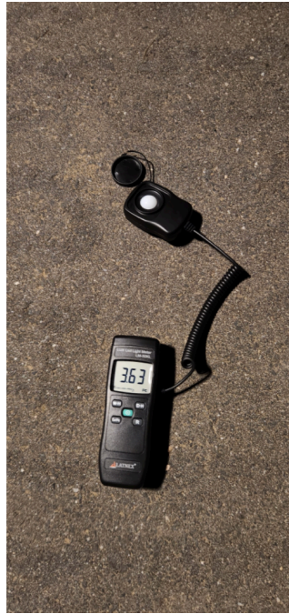
(B) cont. 3.63 FC beneath pole, 0.59 FC between poles, respectively. (Desired: 0.3 FC).
