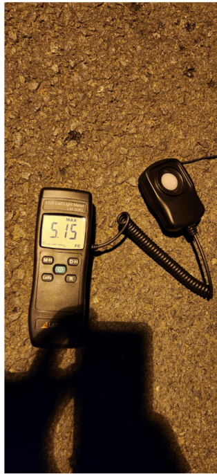
(B) Low post shoebox sodium, very well shielded, slightly overlit. One of the best lighting on campus, even though the backlight is not desirable at other parts of Faculty Rd. Closer to Broadmead. 5.15 FC directly beneath pole, 0.81 FC between poles, respectively.
