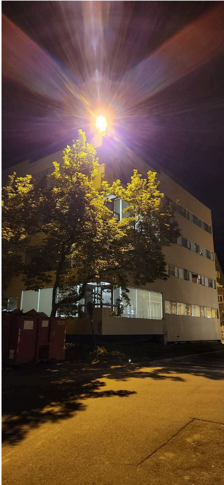
(C) Strong spotlight glare from top of building, majority of light being blocked by top of tree, creating dark patches beneath and blinding passersby.
