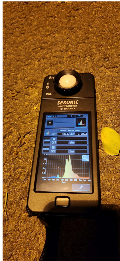
The spectrum peaks around 610nm, corresponding to a color temperature of 1970K.
