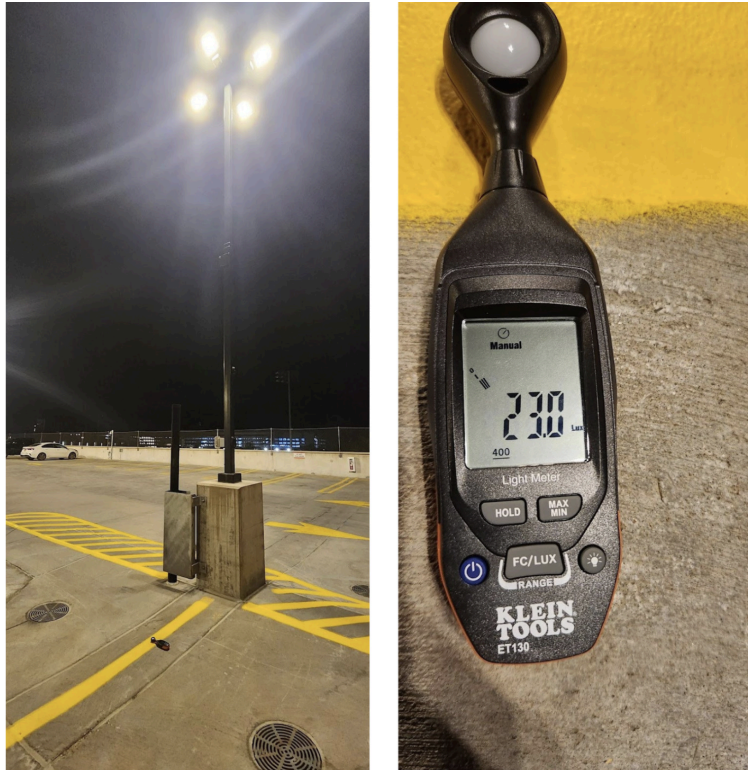
(B) Roof of Stadium Garage, directly beneath pole, 2.3 FC reading (convert from lux).
