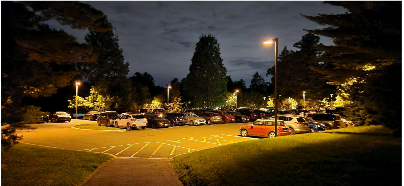
The Graduate School parking lot. Illumination levels are slightly above specs, but light spills out due to non-perfect shielding.
