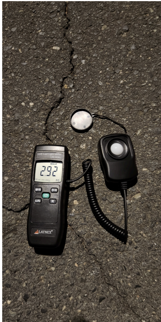
(A) These are low post LEDs with ~3000K light, 2.92 FC directly beneath pole, 1.6 FC between poles at the center of the street. (Desired value 0.3 FC).
