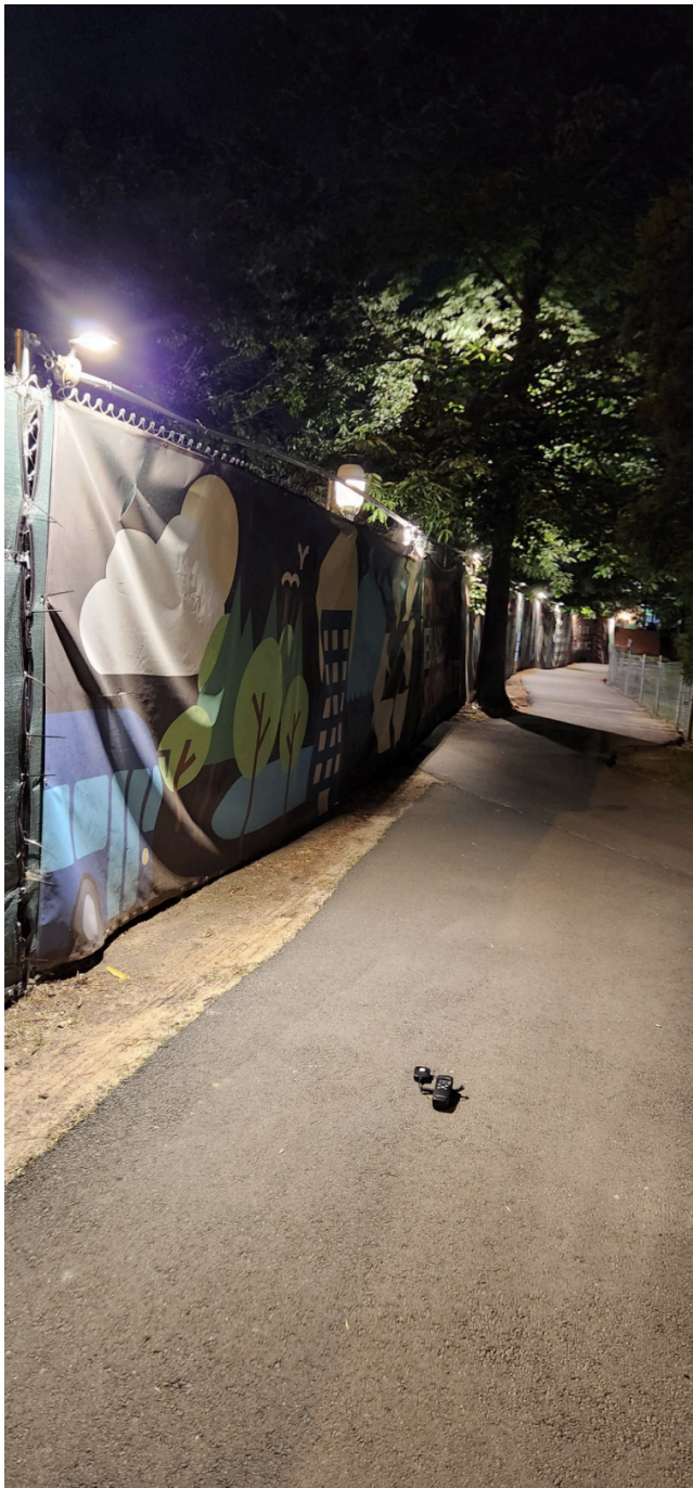
(D) Makeshift LEDs for the walkway. Extremely bright, causing the loss of dark adaptation for other areas that are ~ 10x less lit, 12.77 FC measured.
