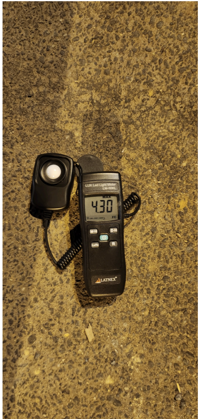
(B) Strong area lights from the top of the building, causing glare and overlighting, 4.3 FC measured. (Desired value 0.3 FC).
