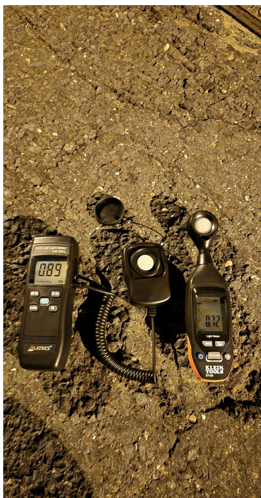
(B) College road, roadway lighting, sodium, lower estimate. 5.7 FC under post, 0.9 FC between posts. (Desired: 0.3–0.6 FC)
