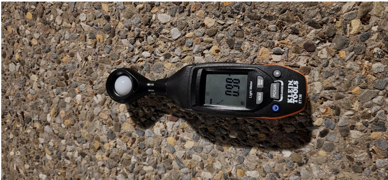
(C) Illuminance measurements on Stadium Drive's walkway, halfway between light fixtures. The reading is 0.98 FC.
