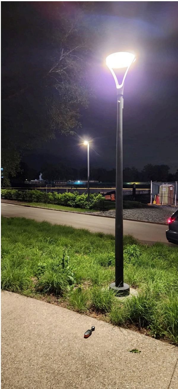
(C) Illuminance measurements on Stadium Drive's walkway under the light fixture. The reading is 3.92 FC; the walkway is overlit by factors of many.
