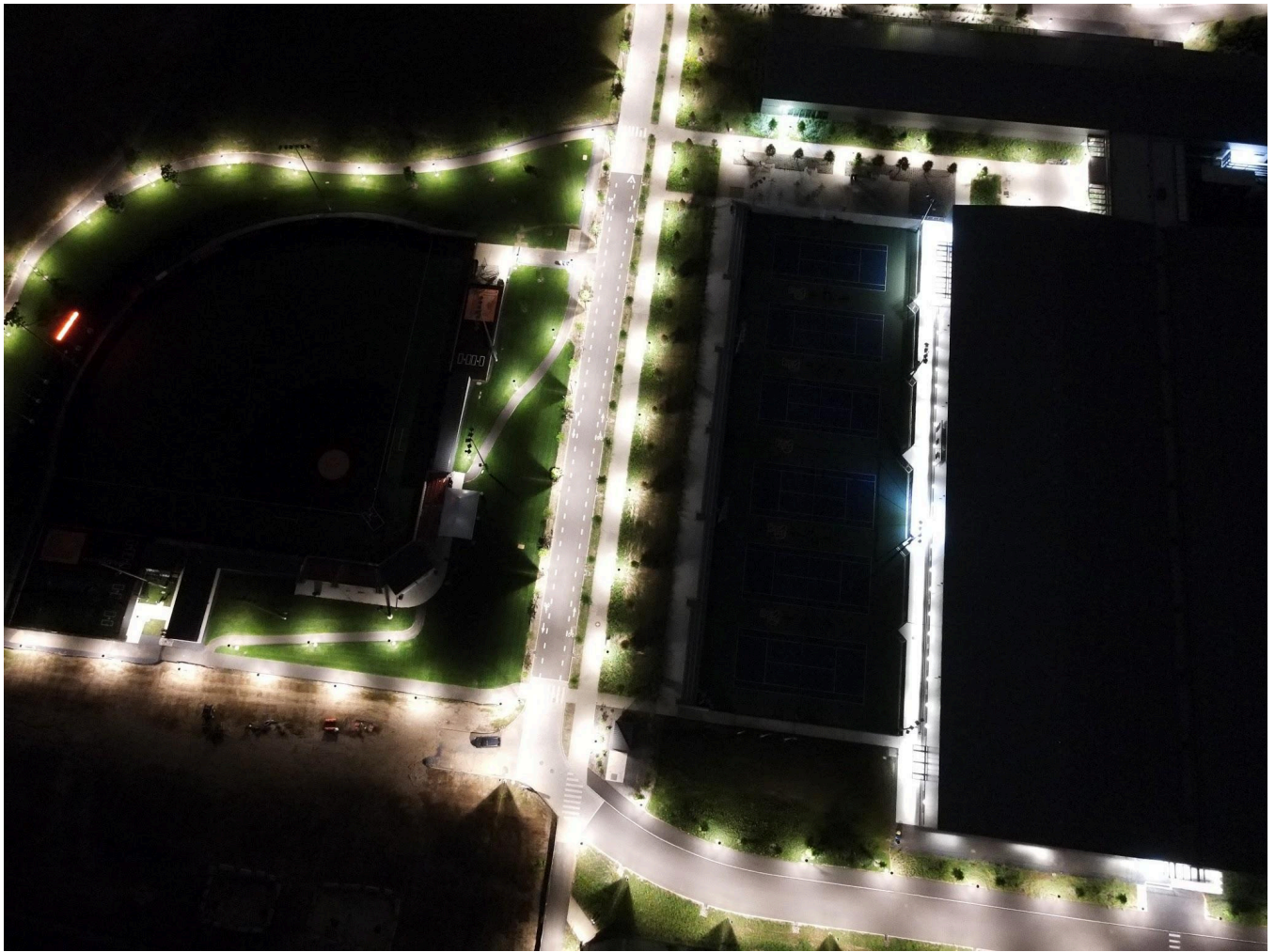
The central alley of the Lake Campus with sidewalk and roadway lights combined, yielding an overlighting of a factor of ~5. Lighting on the edge of the tennis courts with strong vertical light leakage.
