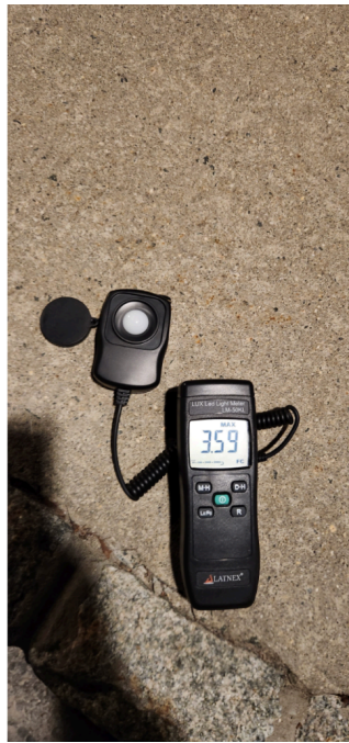
(A) Shoebox LEDs on high poles. Generally overlit, and the lighting is homogenous due to the high poles. 3.59 FC directly beneath the pole and 2.15 FC between the poles, respectively. (Desired value 0.3 FC).
