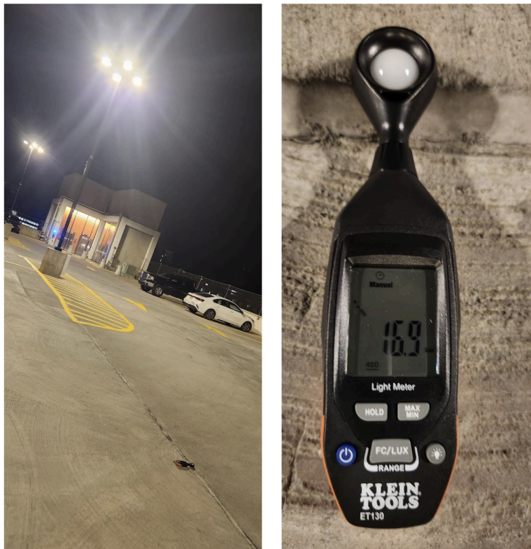
(B) Measurements of the horizontal illuminance on the roof of the Stadium Drive Garage, halfway between lamp posts. In this measurement, the light meter was set to “Lux” units, where 1 Lux is approx 0.1 FC; thus, the readings should be divided by 10 to get values in FC.
