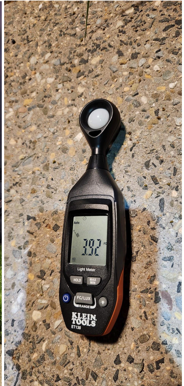
(C) Illuminance measurements on Stadium Drive's walkway under the light fixture. The reading is 3.92 FC; the walkway is overlit by factors of many.
