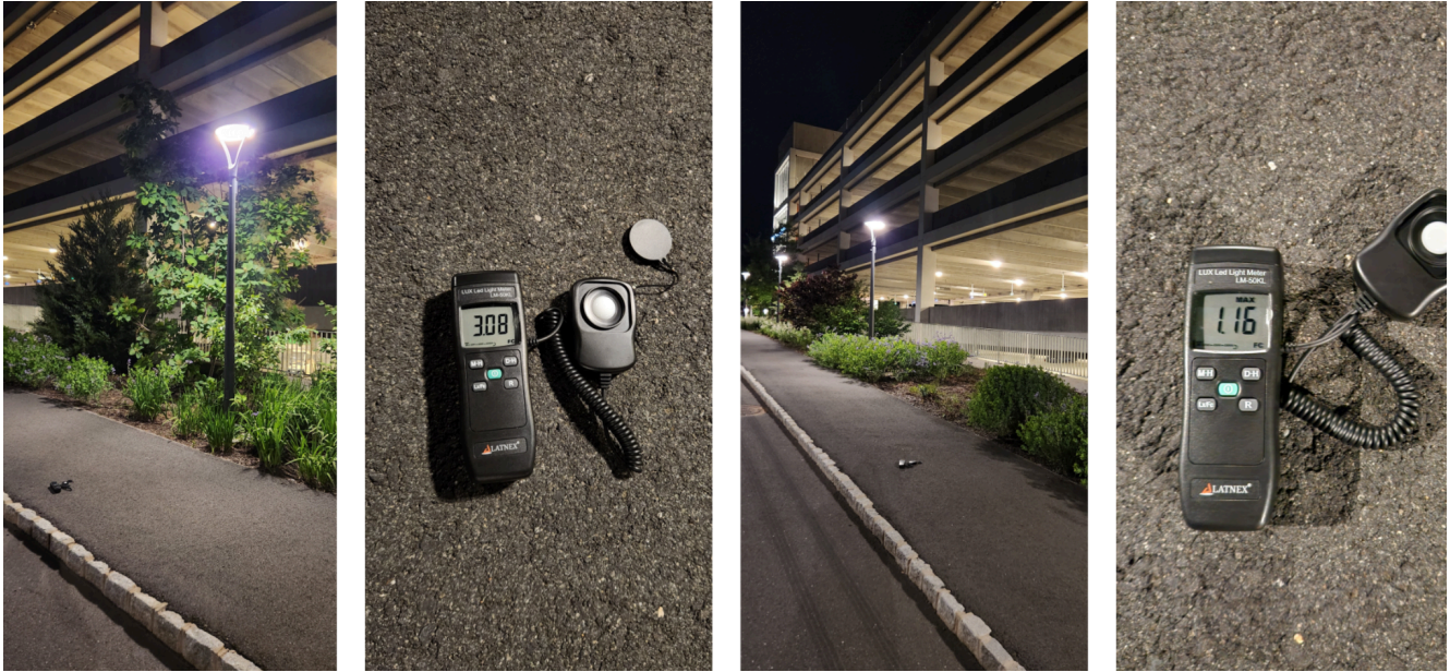
(A) Light measurements beneath & between poles on the walkway near Stadium Garage, 3.08 & 1.16 FC respectively.
