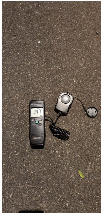
(E) The walkway is excessively illuminated, with both roadway and sidewalk fixtures operating at light levels far higher than necessary, 3.47 FC beneath the pole and 1.66 FC between poles, respectively. (Desired 0.3 FC).
