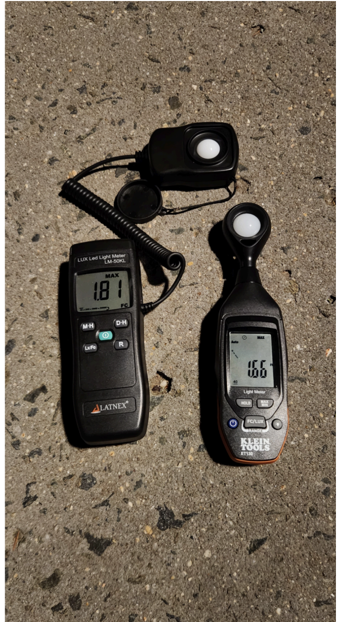
(C) Path from parking lot to graduate college, Penn globes, brighter beneath post, lower but still acceptable limit between posts. Light spills into the nature area. 1.81 FC & 1.66 FC measurements with two different detectors to check for consistency.
